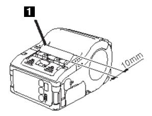
**Note:** When using non-separate labels, press the FEED button to feed a piece of label and pull the label upward to cut it along the perforation. If the label becomes jammed, retry the label setting procedure.
